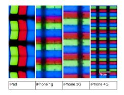
Figure 2: Pixel densities have improved for each succession of the iPhone. The iPad tablet has a lower resolution because operating distance is larger.
